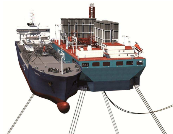
A 25,000 m 3 FSRU with a 20,000 m 3 shuttle tanker
